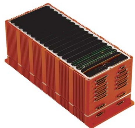
Figure 2 - Standard Housing with cover removed reveals individual card shielding
