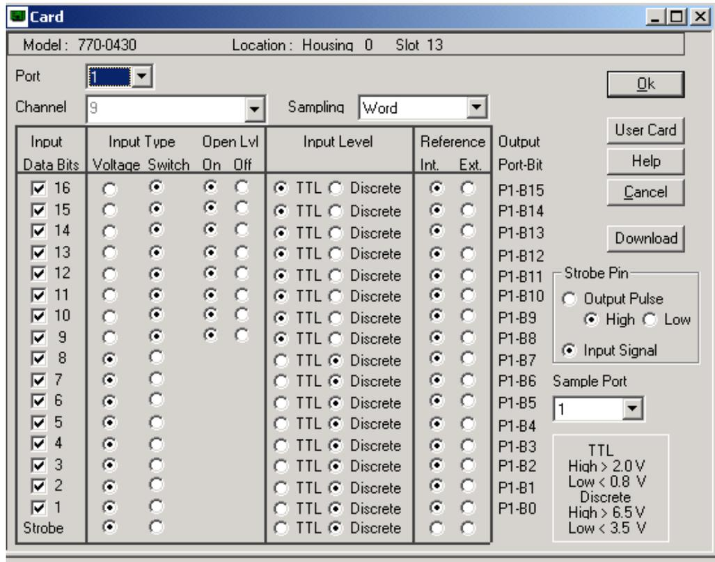
This Bilevel Multiplexer card has the ability to detect sixteen events, which can be independently assigned to four different card ports for insertion into the PCM output. Each port can be sampled independently by PCM channel word or synchronously by frame sync, port, or external strobe input. The strobe pin is programmable as an input for externally latching bilevel data or as an output for use by customer equipment.
