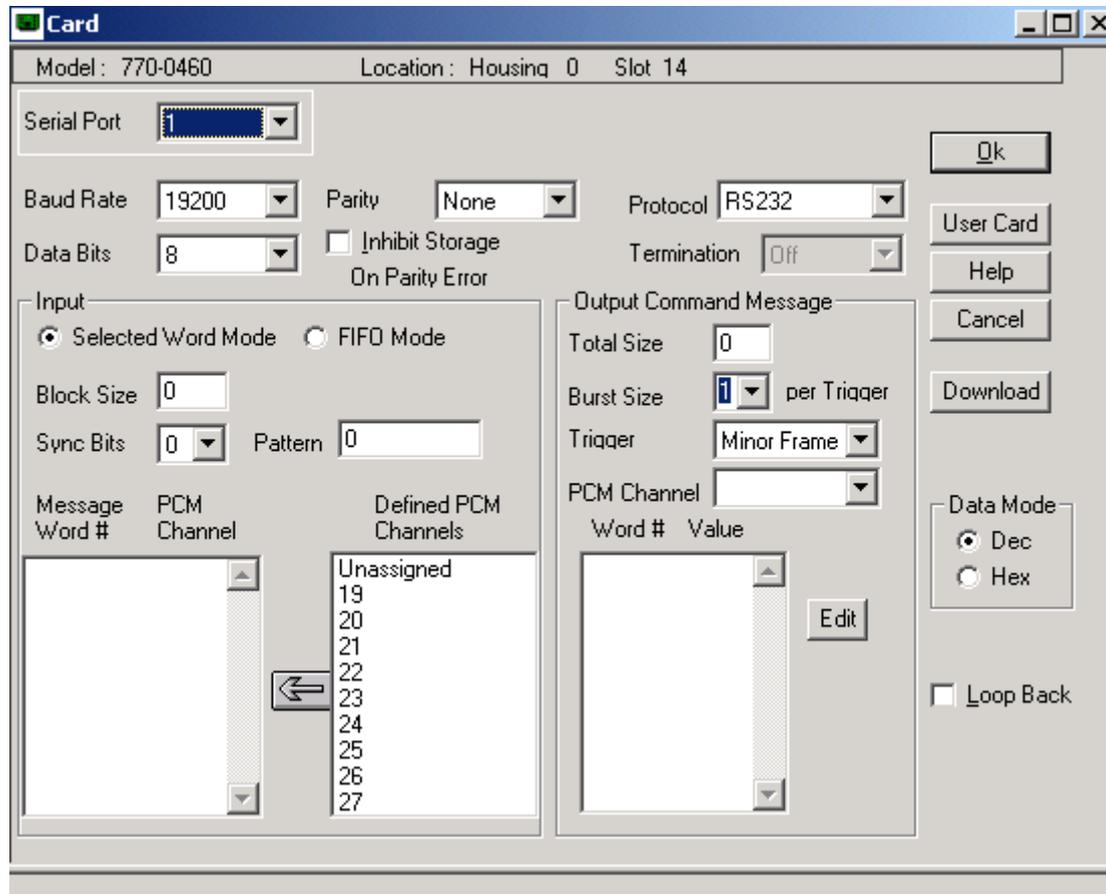
The Serial Interface Card accepts RS-232, RS-422, or RS-485 input data and formats it for insertion into the PCM stream. Each interface can be programmed to search for various synchronization and identification labels and to capture up to 512 selected data words. If desired, all data can be captured and assigned to one PCM channel as an IRIG 106-96 asynchronous data channel. Each interface can transmit up to 128 command words to initiate communications with customer equipment.
