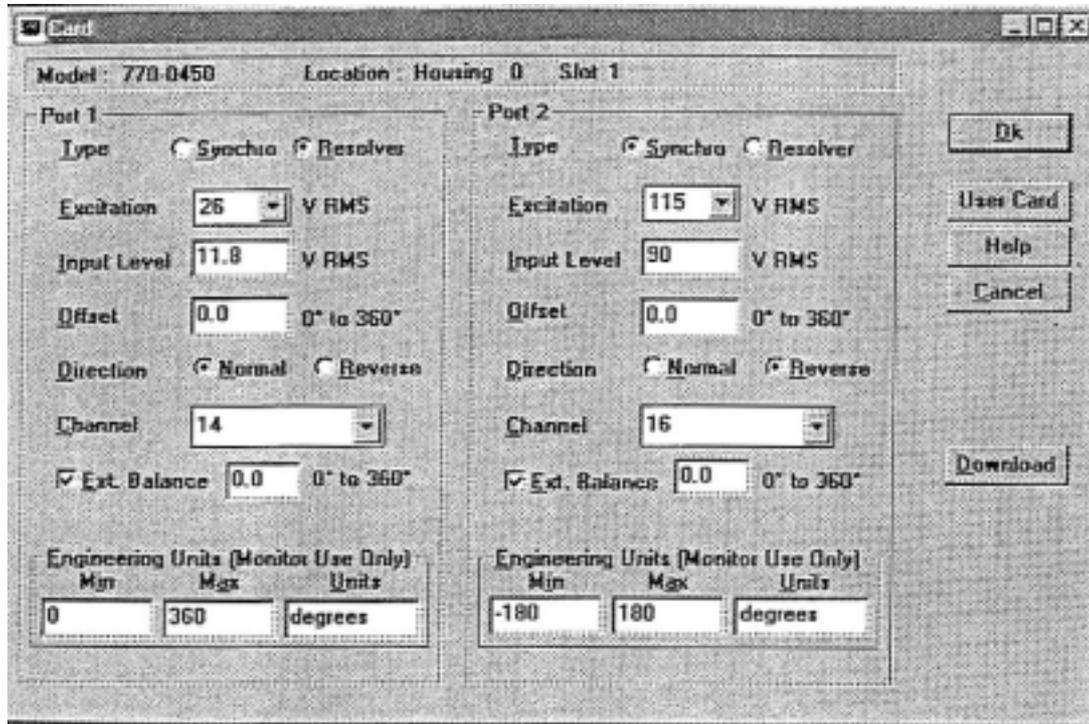
The Dual Synchro/Resolver Card converts 5-wire synchro or 6-wire resolver inputs to 16-bit digital words. Each card has two converter channels. Each channel is independently programmable for either synchro or resolver operation. Input reference and input signal voltages are programmable for industry standard values.
