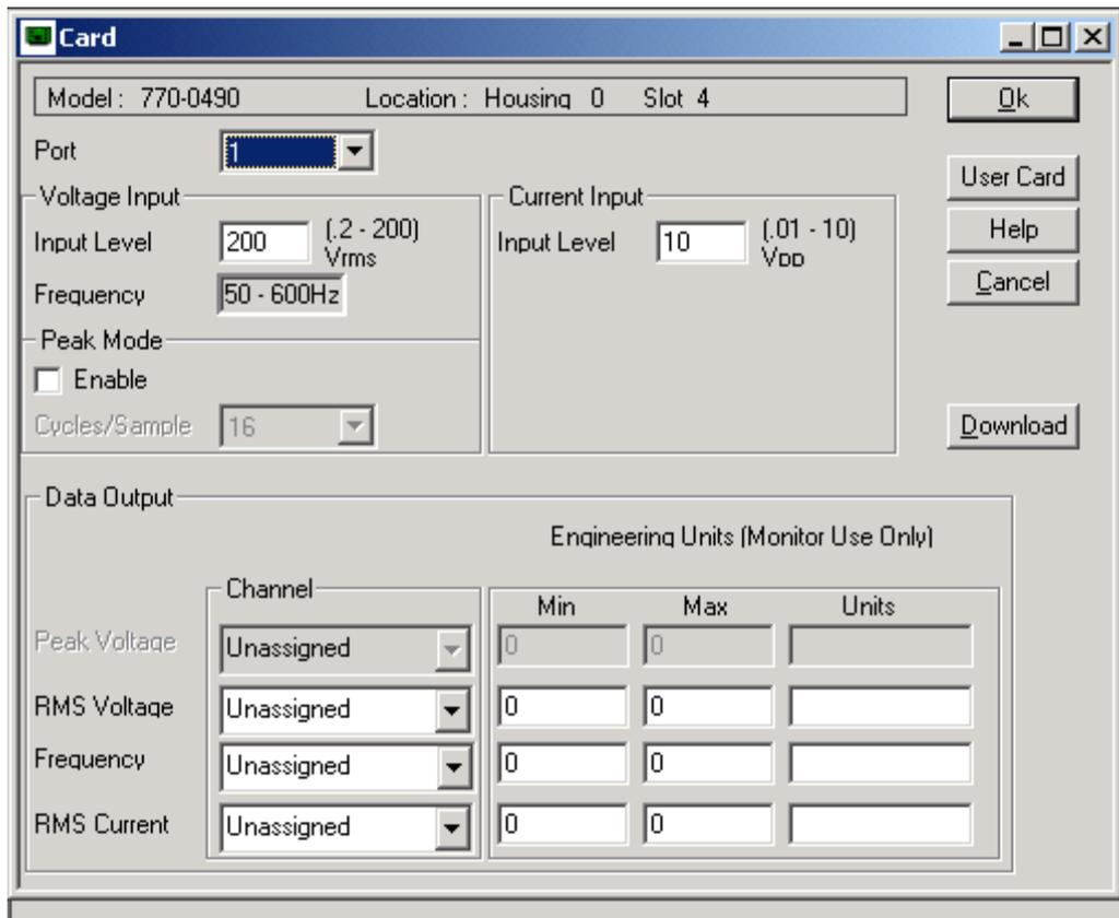
The AC Monitor Card is designed to monitor the AC power voltage and current buses of the system under test. Each channel has an independent multiplexed analog to digital converter (ADC), and separate inputs for monitoring current and voltage.
