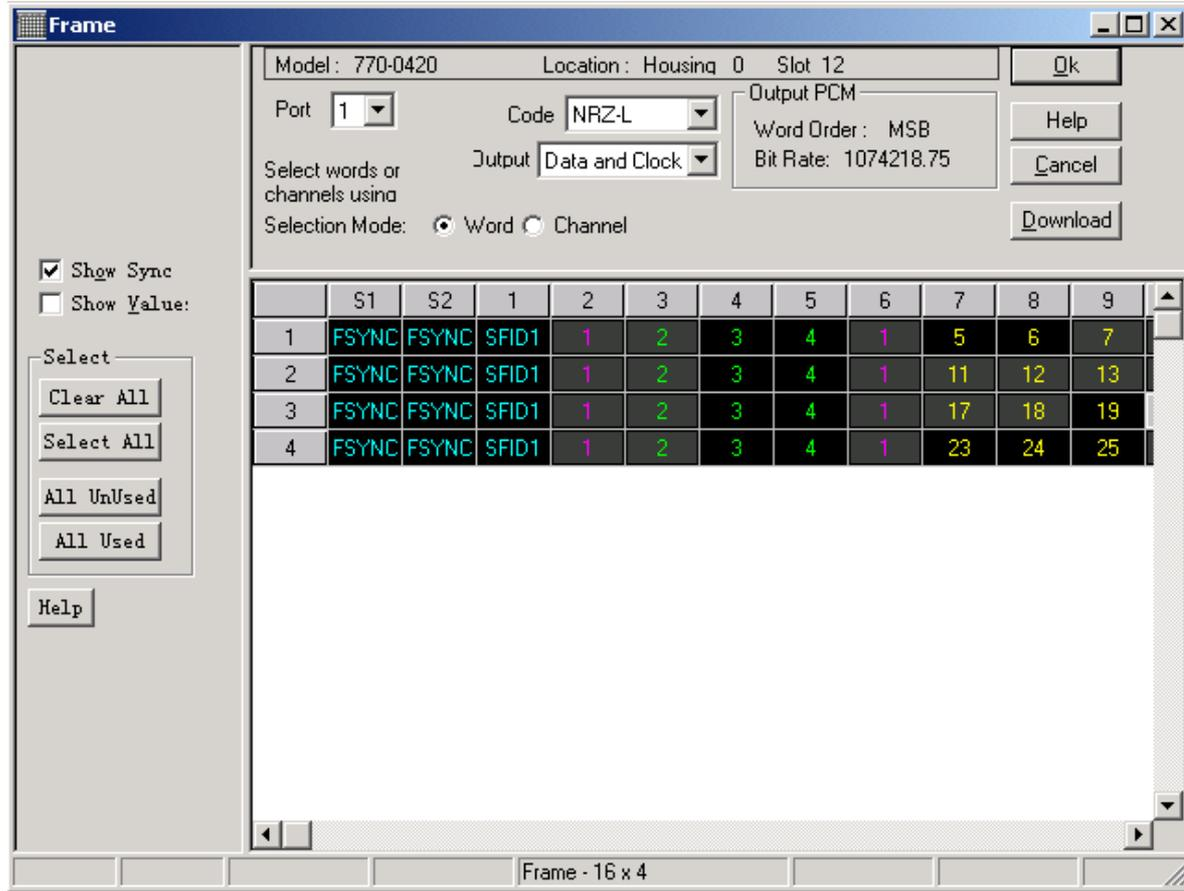
The Selected Word PCM Output Card has the ability to select an entire frame for output at the same bit rate or to select specific words for output at a submultiple of the bit rate.
