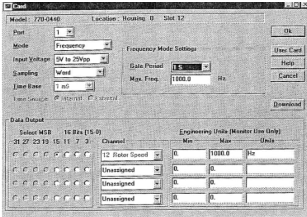
This card is a universal pulse measuring card device with two independent channels for measuring pulse frequency, period, time, mark time, and totals with 32-bit capacity. All functions are user programmable, including the internal time base.
