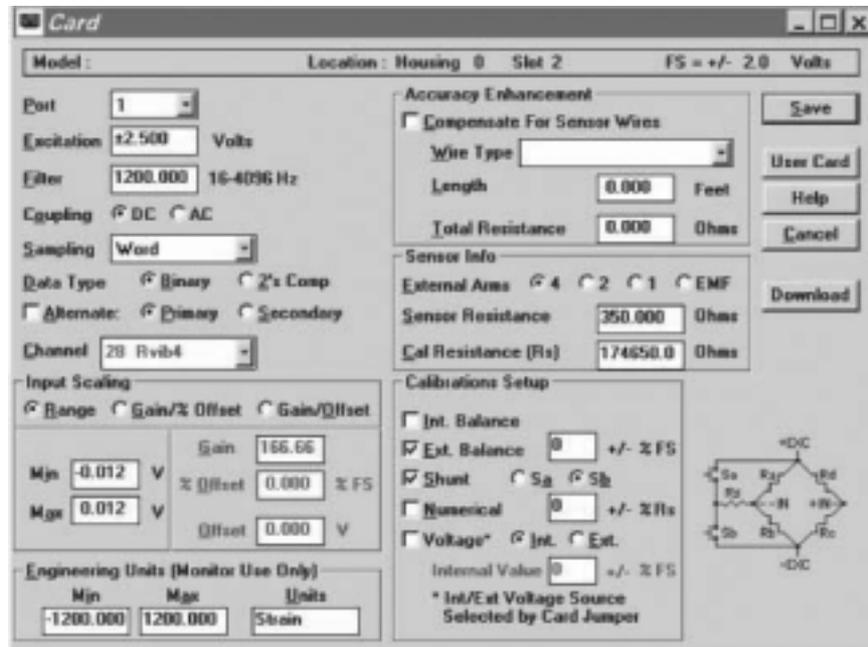
Universal Bridge signal conditioners are designed to interface to 1, 2, or 4 external arm resistive bridges, potentiometers, or other transducers that require a voltage excitation source and provide a voltage output to be amplified, presample filtered, or digitized prior to insertion into the PCM stream.
