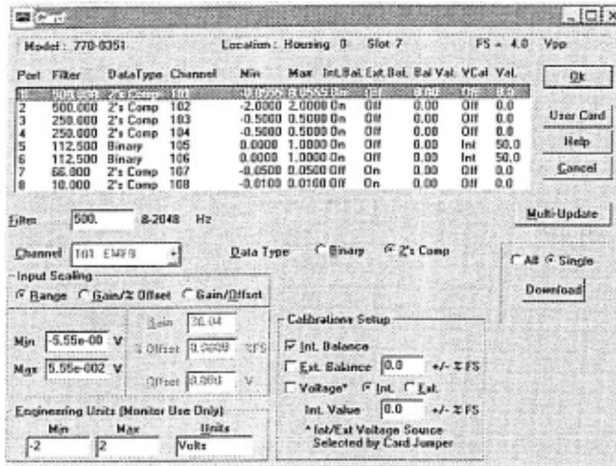
CMV EMF signal conditioners are designed to accept common mode voltage (CMV) electromotive force (EMF) inputs from high impedance voltage sources. CMV EMF signal conditioners are available in two input voltage ranges; Low range (4 Vspan) and High range (100 V span).
